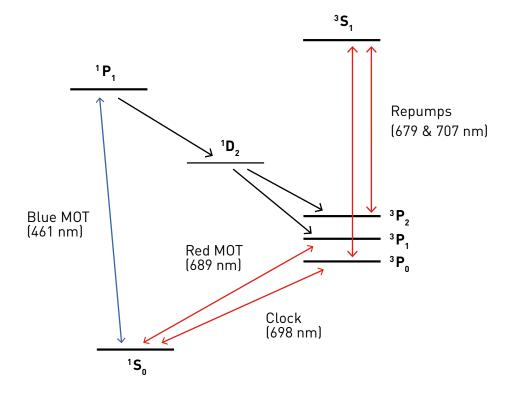
The second stage (red MOT) uses light at 689 nm to further cool atoms down to temperatures on the order of a micro-Kelvin.
